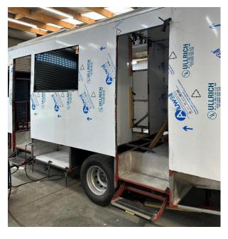
Vehicle closed in, note 55-inch TV in place built into the side of the vehicle. Protective paper over the aluminium sides
